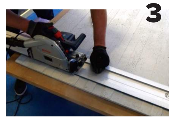
— START CUTTING WITH A PLUNGE-CUT SAW
